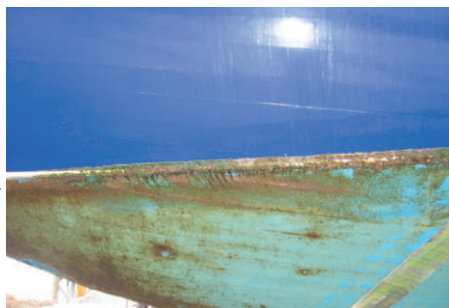
Portside forward end: weed on the waterline and slime below... The power washer takes all the slime off... The finished job; ready for another season
