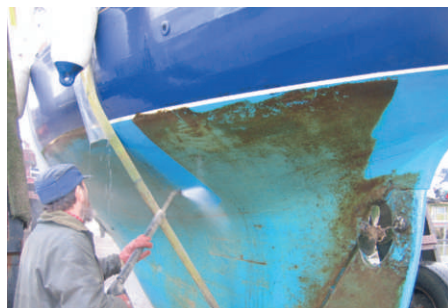
Portside forward end: weed on the waterline and slime below... The power washer takes all the slime off... The finished job; ready for another season
