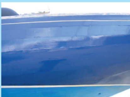
This area takes the worst of the weather, but the paint hasn't broken away and is giving some protection to the seams
